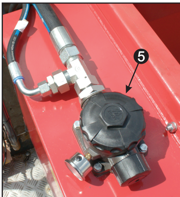
Photo 25 - Hydraulic tank return filter
